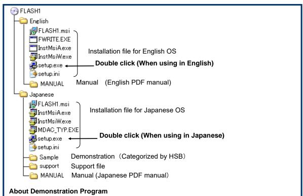
Attached CD also includes the sample program for HSB series MCU board by HokutoElectronicd. In "sample" folder of the CD, there are 4 programs for each MCU type; freqmeta.mot, stopwat.mot, voltmeta.mot, watch.mot. Please note that all these programs are in Japanese. All comments will be displayed correctly with Japanese OS>
